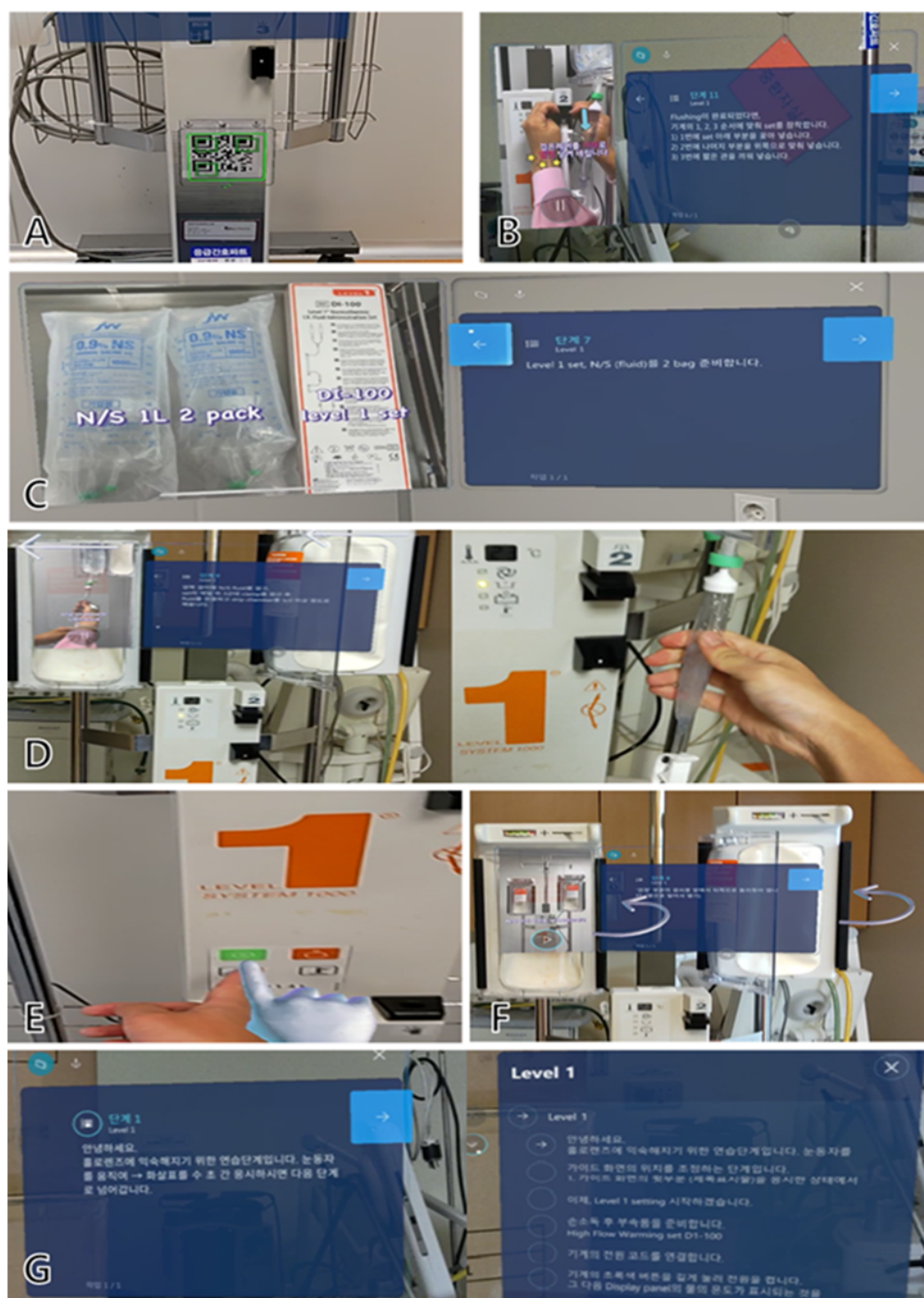
Figure 1. Trainee's view during augmented reality-based training for the Level-1 rapid infusion system. (A) The anchor affixed to the device retrieves prestored instructional content and serves as a spatial reference for hologram positioning. (B) Finger-shaped holograms guide users to button locations. (C) Required materials for each step are displayed in advance. (D) Learning objectives appear in a blue instructional window. (E) Short instructional videos are played as holograms for complex operations. (F) The trainer's hand movements are displayed for procedures that require visual demonstration. (G) The step navigation interface: a practice card that advances to the next step when the trainee gazes at the arrow (left) and the expanded step list for the Level-1 setup procedure (right).
