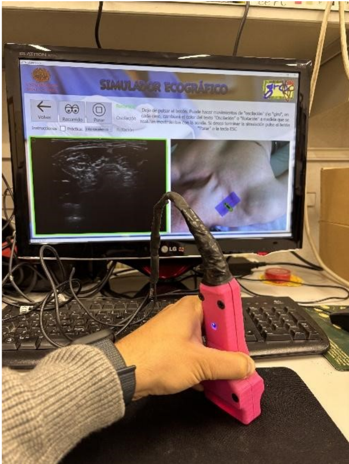
Figure 1. Illustration of the probe's movements as recorded by the software, which are used to enhance the precision of the ultrasound-guided approach.
