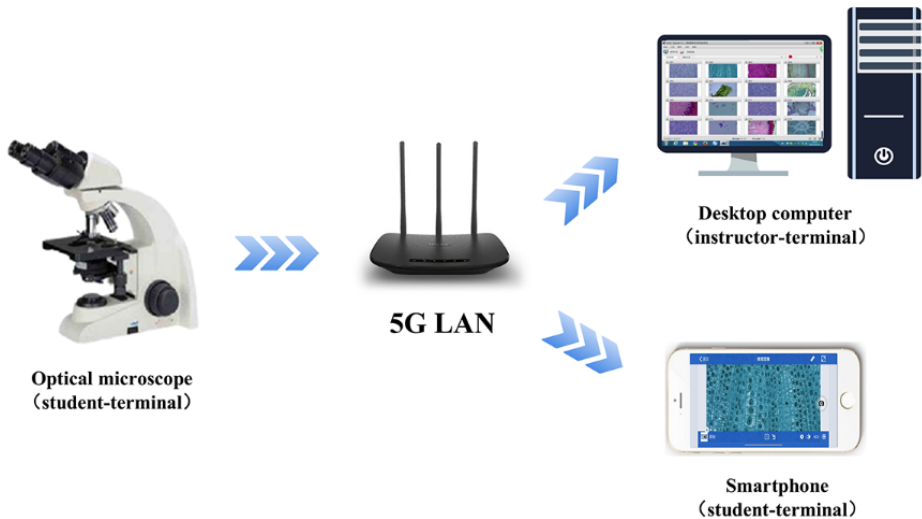
Figure 1. The framework of a digital microscopy interactive system based on 5G local area network (LAN).
