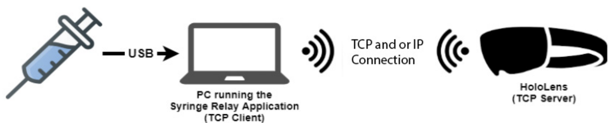
Figure 2. The sequence of communication between the potentiometer and HoloLens. Note that the potentiometer is embedded within the syringe displayed at the left. TCP: transmission control protocol.
