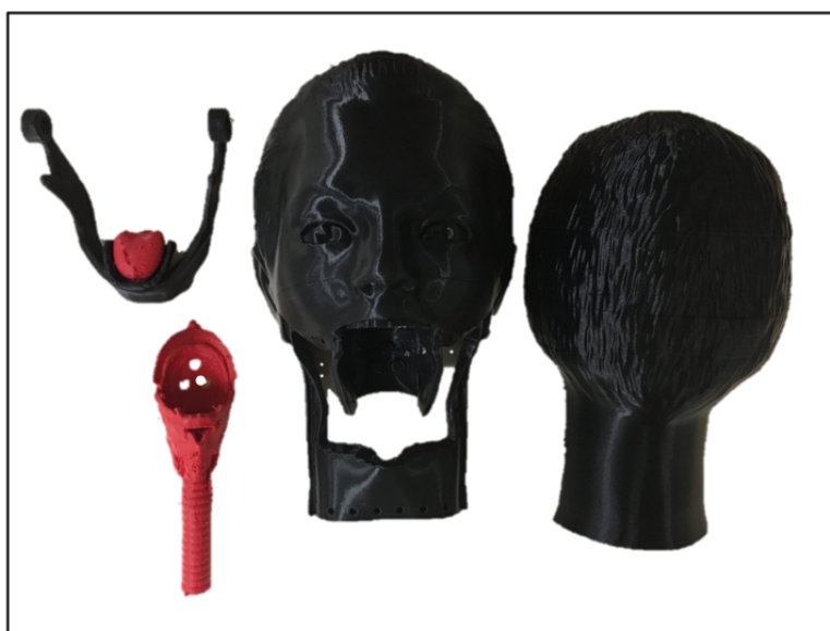
Figure 7. Three-dimensional–printed pieces from left to right: mandible and tongue, throat, head coronal cut 1 and 2. Dimensions: 25.5x16x21 cm.
