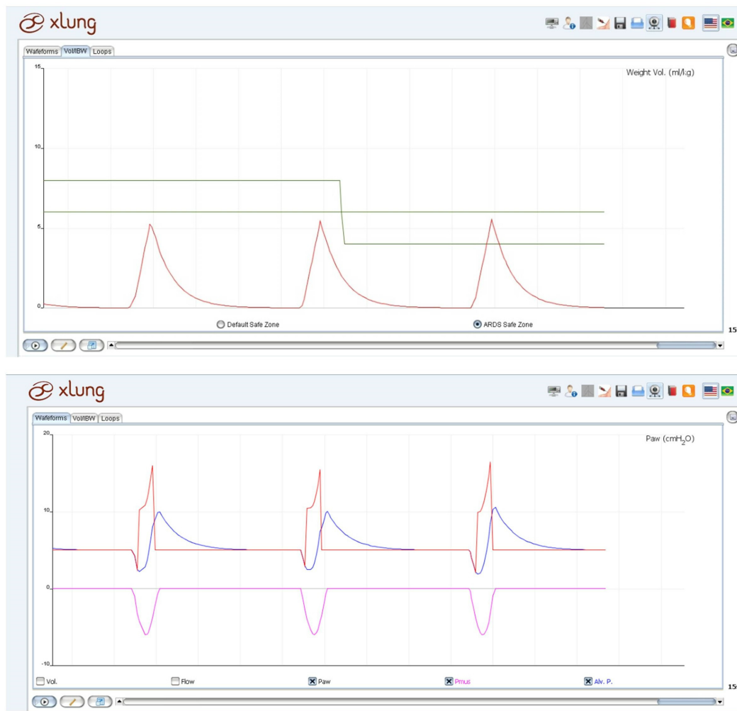
Figure 3. Special graphics of the Xlung MVVS. At the top, ponderal tidal volume according to the ideal body weight (mL/kg) with depicted safe zones and at the bottom, exhibition of airway (red), muscular (pink), and alveolar (blue) pressures altogether.
